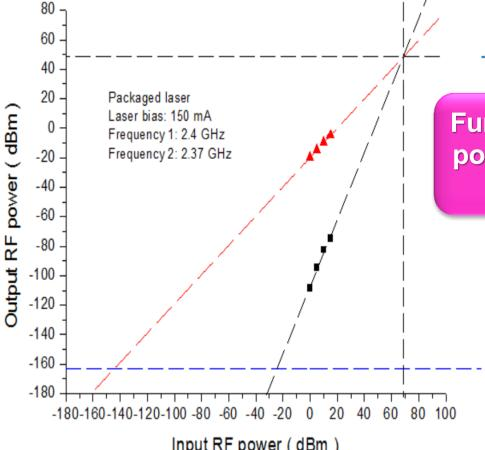
Fundamental and IMD3 RF output powers as a function of input RF power at 2.4 GHz
